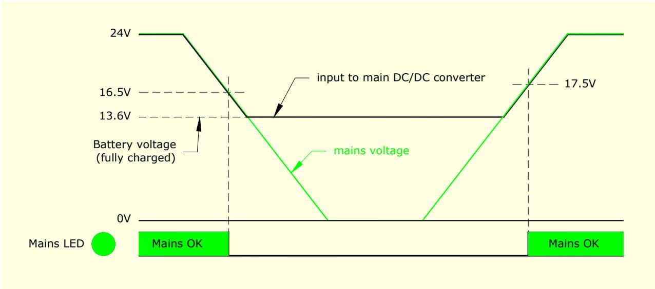
The connected lead-acid backup battery is maintained by an integrated battery charger (fast charge and trickle charge). Using an external battery temperature sensor, you can disable the charging if the battery is too hot. See the section *Battery monitor and charger*.
