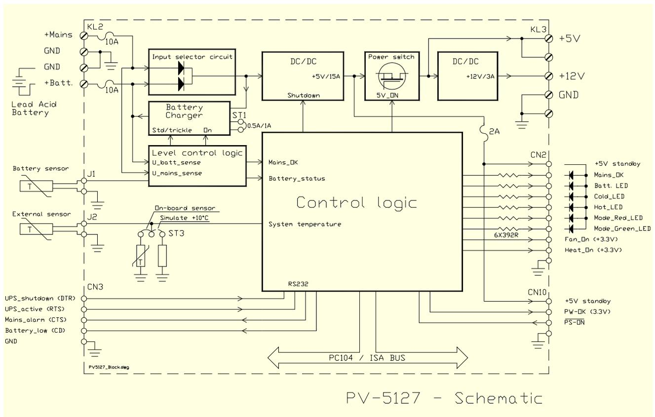
PV-5127 is built around a high efficiency DC/DC converter that converts the incoming DC voltage to 5V/15A. This output is used for +5V Standby and is available at CN2 and CN10. A power switch is used for turning on/off the output voltages +5V and +12V under software control and by the safety shutdown function.
