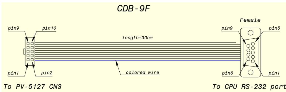
The signals use normal RS232 voltage levels. Inactive (‘0’) = -10V, active (‘1’) = +10V. In the table shown inputs are indicated by (i) and outputs by (o).
