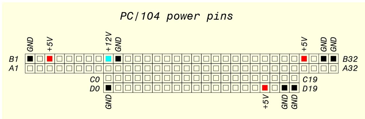
The ATX signals (+5V STB, PS\_ON and PWR\_GOOD) are not available in the PC/104 connector. The PC/104 bus is also used for software UPS status and power-off, see the *UPS Control* section. The software interface uses the following signals:
