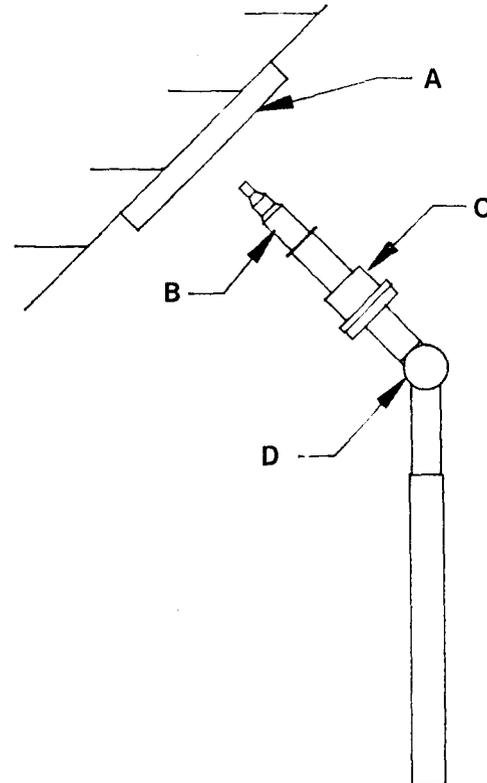
The sloped ceiling adapter is now ready for insertion of Focal Jacks or Extender Stems.
