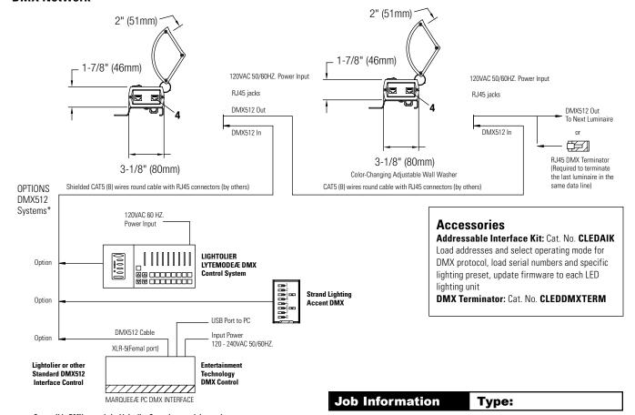
Compatible DMX controls by Lightolier Controls www.lolcontrols.com
