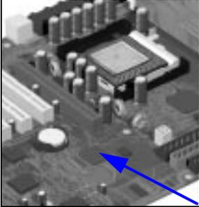
The ICH2 is encapsulated in a 360-pin Enhanced Ball Grid Array (EBGA) package and is located on the system board just underneath the AGP connector. It provides the interface between the PCI bridge (PCI Rev. 2.2 compliant with support for 32-bit 33 MHz PCI operations), PCI-to-LPC (Low Pin Count) bridge, IDE controller, USB controller, SMBus controller and Audio Codec '97 controller.
