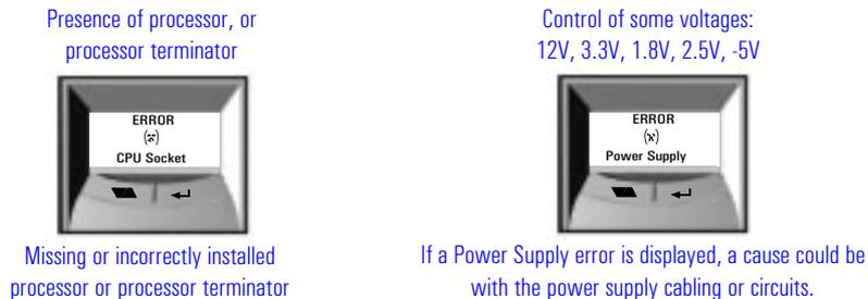
The following diagram shows how the Pre-boot Diagnostics works when it encounters an error.
