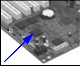
MaxiLife is a hardware monitoring chip which is resident on the system board. Its responsibility includes On/Off and reset control, status panel management (Lock button, LEDs), hardware monitoring (temperature and voltage), early diagnostics (CPU, memory, PLLs, boot start), run-time diagnostics (CPU errors), fan speed regulation, and other miscellaneous functions (such as special OK/FAIL symbols based on a smiling face).
