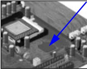
The MCH Host Bridge/Controller is contained in a 615-pin Organic Land Grid Array (OLGA) package and is the bridge between the System bus, Dual Rambus bus (main memory), AGP 4x (graphic) bus and Hub Link 8-bit.
