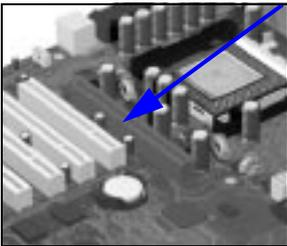
Minitower models of the HP Kayak XU700 are equipped with a single AGP (Accelerated Graphics Port) graphics slot.
