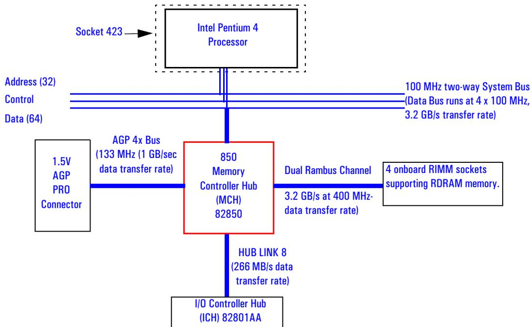
The supported operating frequency of the GTL+ bus for the Pentium 4 is 100 MHz. The width of the data bus is 64 bits, while the width of the address is 32 bits. Data bus transfers occur at four times the system bus, at 400 MHz. Along with the operating frequencies, the processor voltage is set automatically.
