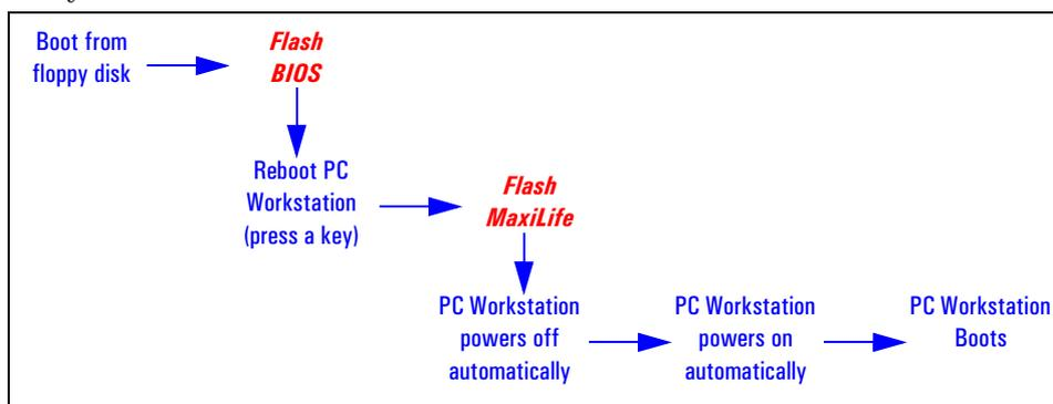
Do not switch off the computer until the system BIOS update procedure has completed, successfully or not, otherwise irrecoverable damage to the ROM may be caused.
