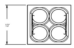
Complete fixture consists of Reflector Trim (4 needed), Frame-in Kit and Face Plate. Select each separately
