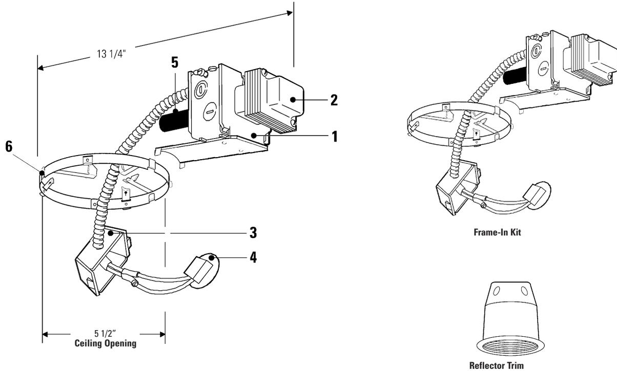
Complete Fixture consists of Reflector Trim & Frame-In Kit. Select each separately.
