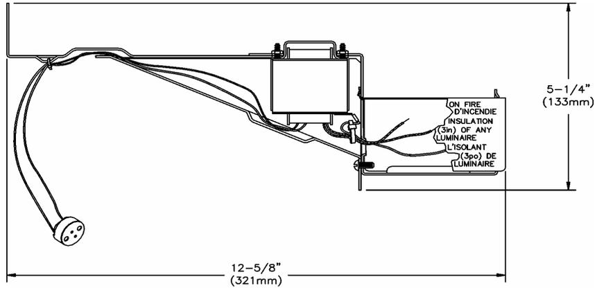
Complete fixture consists of Reflector Trim & Power Pack. Select each separately
