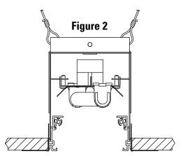
Provide Power to Fixture Through Access Plate and Test. Build Ceiling Around Fixture Then Fasten Corner Bead material to Ceiling and Finish Ceiling.
