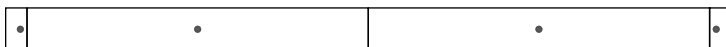
16' Run: 8' (243.84cm) Master Module, 8' (243.84cm) Slave Module, Single Sensor End Set, and Intermediate Cable Assembly.
