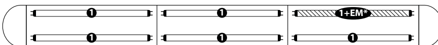
All lamps wired on one circuit, plus a battery pack is wired to one lamp. A hot lead is connected to the battery pack and would function as a 'trigger' wire when connected to a constant hot by installer. Leads for both normal circuit and battery pack are wired to fixture ends.
