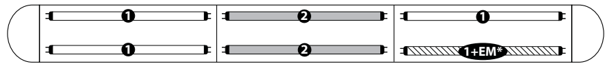
Fixture wired for two circuits (A/B switching), plus a battery pack is wired to one lamp. A hot lead is connected to the battery pack and would act as a 'trigger' wire when connected to a constant hot by installer. Leads for both normal circuit and battery pack are wired to fixture ends.
