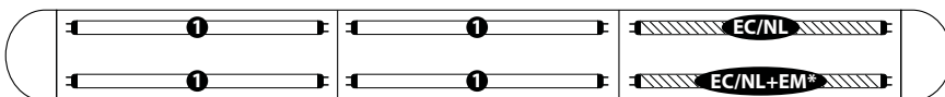
One 4' section in a one circuit fixture to be wired on a separate thru circuit, in addition, a battery pack is wired to one lamp. Installer can connect 'trigger' wire to EC hot lead if controlled together or wire separately if controlled independently. Leads for normal circuit, EC/NL and EM wired to fixture ends. All lamps in EC/NL section to be wired together.
