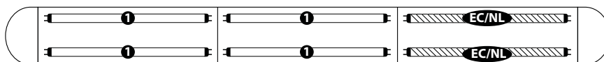
One 4' section in a one circuit fixture to be wired on a separate thru circuit. Leads for both normal circuit and EC/NL circuit wired to fixture ends. All lamps in EC/NL section to be wired together.
