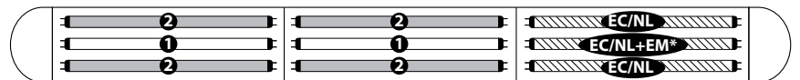
One 4' section in a two circuit fixture (center/outer switching) to be wired on a separate thru circuit, in addition, a battery pack is wired to one lamp. Installer can connect 'trigger' wire to EC hot lead if controlled together or wired separately if controlled independently. Leads for normal circuit, EC/NL and battery pack are wired to fixture ends. All lamps in EC/NL section to be wired together.
