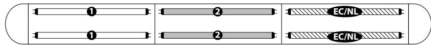
One 4' section in a two circuit fixture (A/B switching) to be wired on a separate thru circuit. Leads for both normal circuit and EC/NL circuit wired to fixture ends. All lamps in EC/NL section to be wired together.
