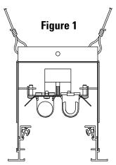
Hang Fixture from Structure Above. Make Sure Fixture is Leveled Lengthwise and Widthwise.
