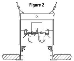
Provide Power to Fixture Through Access Plate and Test. Built Ceiling Around Fixture.
