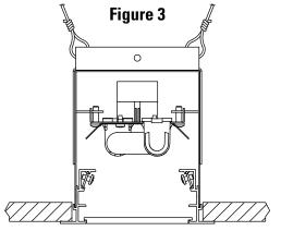
Install Diffuser Provide with Fixture. Lens or Louver.
