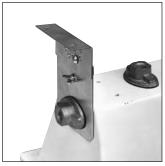
45° ADJUSTABLE STAINLESS STEEL QUADRANT BRACKETS: Two sturdy 'L" type adjusta-mounts with gaskets for field installation at top and side ends of fixture. Permit housing to be permanently surface-mounted and adjusted up to 45° in either direction in 5° increments. Provide wide-spread directed illumination where tasks are not fixed. Specify Bracket Catalog are not fixed. Specify Bracket Catalog Number: NKH45.
