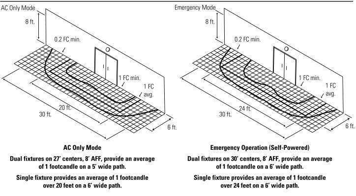
\* The optics layout shown is intended to be used as reference only. Standard reflectances used were 80/50/20. Lightolier is not responsible for site specific conditions that may alter the results.
