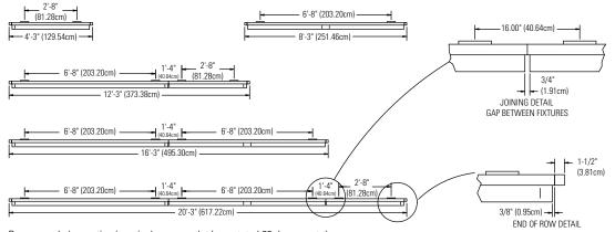
Recommended mounting is a single gang outlet box rotated 90 degrees at the feed point. Remaining mounting points could be outlet boxes as well, or a couple of holes per mounting point spaced 3-1/4" (8.26cm) at 1-3/4" (4.45cm) above the bottom of fixture.
