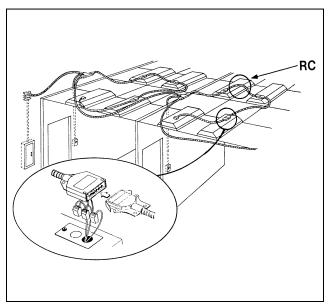
Quick and easy field-installed by plugging ballast leads into "Poke Home" connectors, no wirenuts required.
