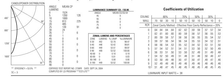
**50W MR16 IR - 40° Flood** GE Halogen Lamp, Lumen Rating = 800 LMS, 120V Electronic Transformer
