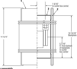
Complete Fixture consists of Lightshield and Backplate Assembly. Order each separately.
