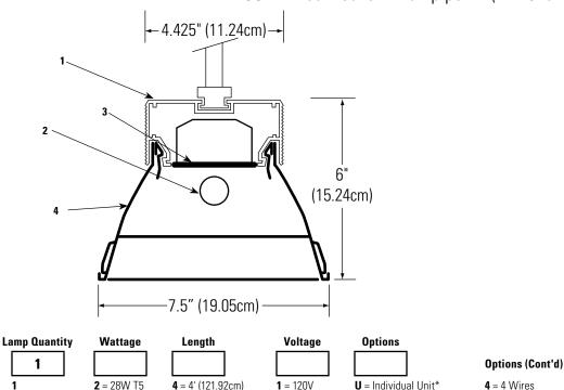
\*Only individual fixtures should use the "U" option. Any fixture ordered without "U" is a joiner for continuous row mounting
