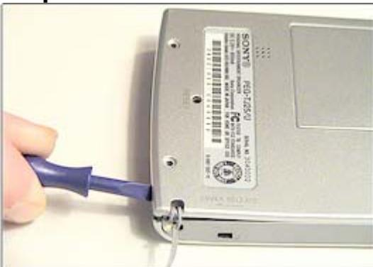
Use the plastic flathead screwdriver or any small flathead screwdriver (plastic recommended - metal may scratch) to separate the back case from the front by CAREFULLY prying around the device. There are clips on all sides of the device holding the front and back together. Be careful not to break them when prying.
