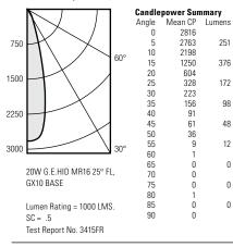
Tested According To IES Procedures. Test Distance Exceeds Five Times The Greatest Luminous Opening Of Luminaire
