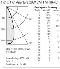
Tested According To IES Procedures. Test Distance Exceeds Five Times The Greatest Luminous Opening Of Luminaire
