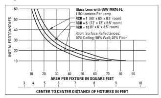
Use quick calculator chart to determine spacing of luminaires for desired level of illumination. Conversion Factors: 37W and 50W MR16 FL: F.C. X 0.7 35W MR16 FL: F.C. X 0.5
