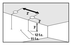
EXAMPLE: With multiple units located 2' from wall and 2' on center, the illumination on the wall 3' down from the ceiling is 12 f.c. beneath and 11f.c. between fixtures.
