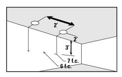
EXAMPLE: With multiple units located 2' from wall and 2' on center, the illumination on the wall 3' down from the ceiling is 7 f.c. beneath and 6 f.c. between fixtures.
