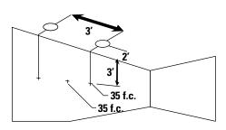
EXAMPLE: With multiple clear reflector units located 2' from wall and 3' on center, the illumination on the wall 3' down from the ceiling is 35 f.c. beneath and 35 f.c. between fixtures.
