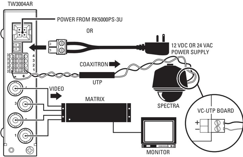
**Figure 6.** TW3004AR Connected to a Spectra Dome
