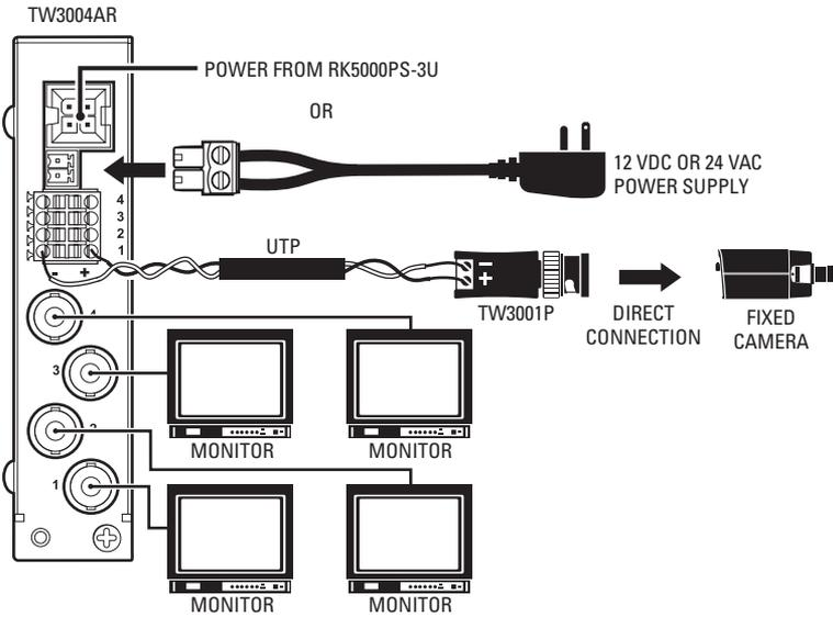
**Figure 7.** TW3004AR Connected to a Single Passive Transceiver
