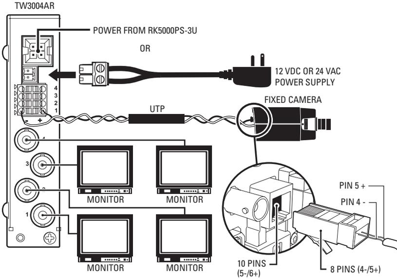
**Figure 5.** TW3004AR Connected to a UTP Fixed Camera
