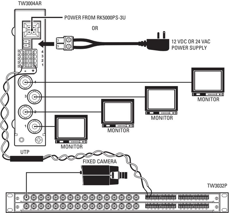
**Figure 8.** TW3004AR Connected to a 32-Channel Passive Transceiver
