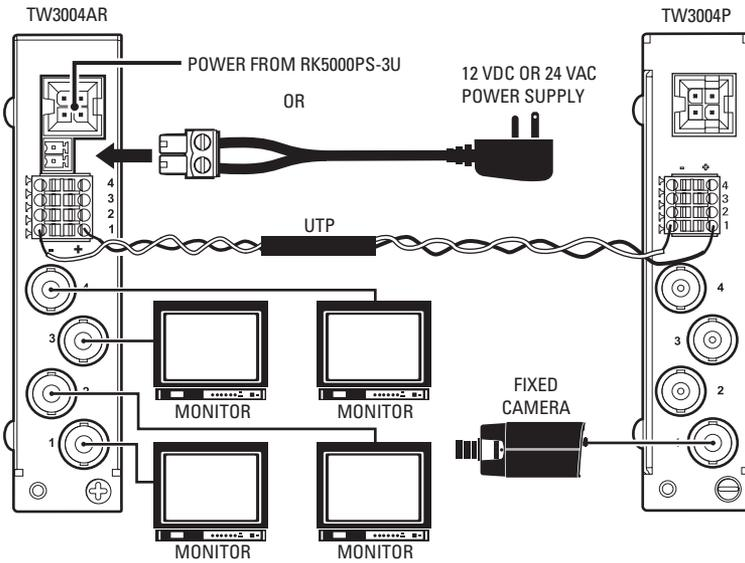
**Figure 9.** TW3004AR Connected to a 4-Channel Passive Transceiver
