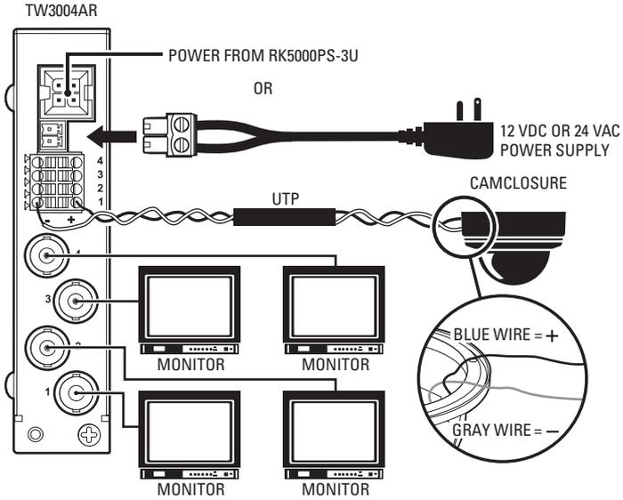
**Figure 4.** TW3004AR Connected to a UTP Camclosure
