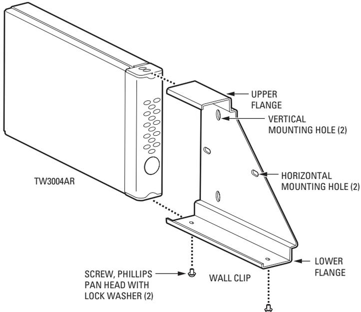
**Figure 2.** Mounting the TW3004AR Using the Wall Clip
