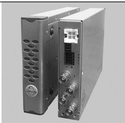
**Four Channels for UTP Transmission**
