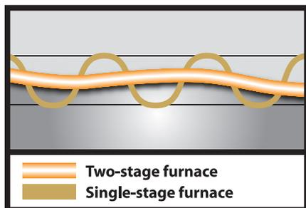
A two-stage furnace can operate at high or low output capacity to accurately and efficiently control home comfort in relation to outside temperature and home heating needs.
