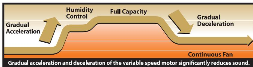
Slow, gradual blower acceleration helps pre-heat the air stream during the heating season and pre-cool during the cooling season, improving overall comfort. The blower-off cycle slowly decelerates, improving energy efficiency year round.
