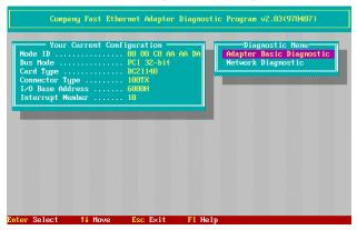
The Configuration Data screen also features a Diagnostic Menu. Follow the cues at the foot of the screen to select and run the Adapter Basic Diagnostic program. The adapter function test results will appear onscreen.
