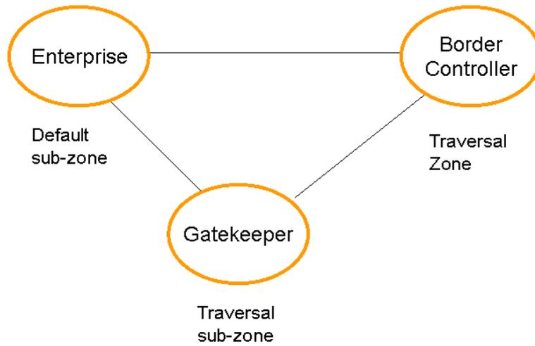
Figure 11: Gatekeeper example configuration
