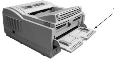
3. Pull down the manual feed tray (1) and adjust the paper guides to the width of the paper.
