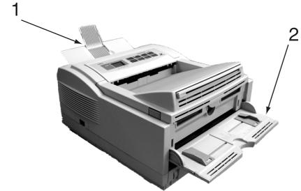
2. Pull down the manual feed tray (2) and adjust the paper guides to the width of the envelope.
