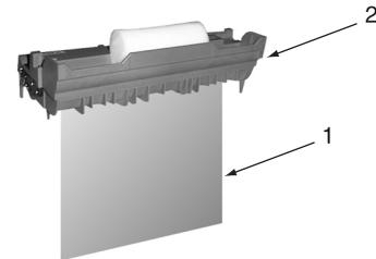
3. Install the new image drum (1) into the printer placing the alignment pins on each end into the slots in the printer.
