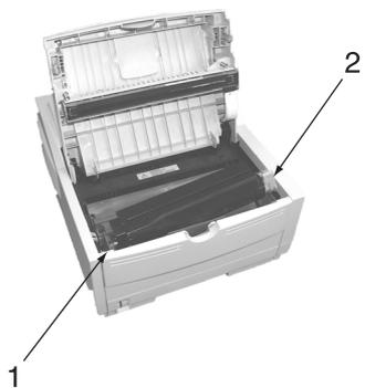
4. Insert the cartridge into the printer, left end (1) first as illustrated.
