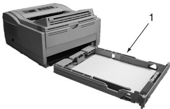
3. Check that the rear paper support has not moved from its paper size setting.
