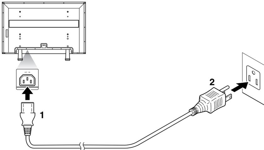
**1** Connect the power cable to the plasma display first.
