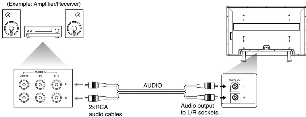
Connect the AUDIO OUT from the plasma display to the AUDIO IN on the amplifier/receiver.
