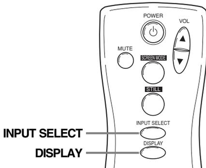
The procedure for selecting the input signal described here is for use with the remote control. However, the **INPUT SELECT** button on the plasma display can also be used in the same way.
