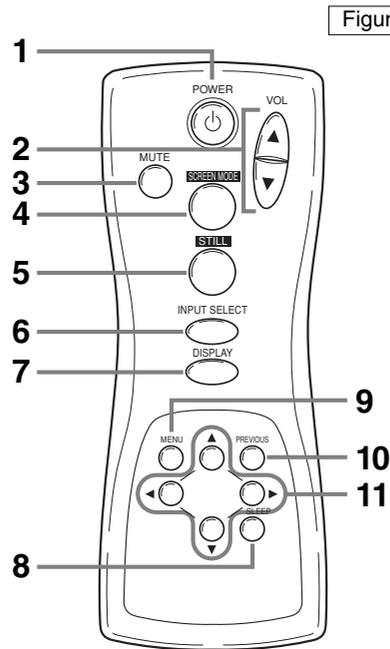
**1 POWER button:** Turns the main power ON or in STANDBY.
