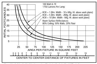
Use quick calculator chart to determine spacing of luminaires for desired level of illumination Conversion Factors:
