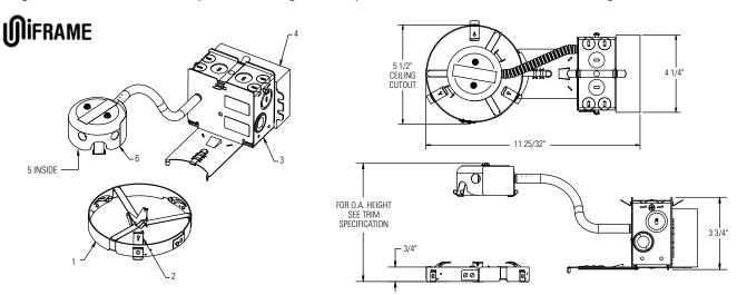
Complete Fixture consists of Frame-In Kit and Reflector Trim. Select each separately.
