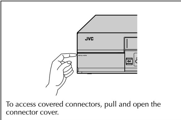
To access covered connectors, pull and open the connector cover.
