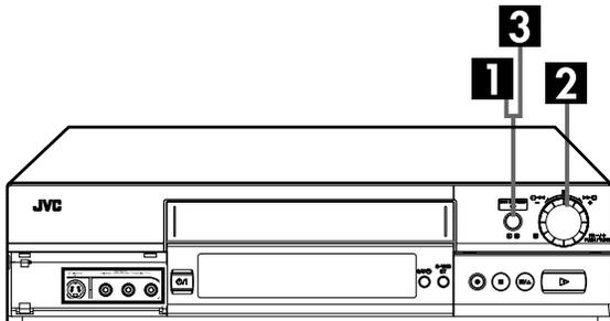
You can programme a timer recording that starts within 24 hours using the JOG dial on the recorder.
