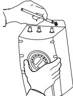
Tank must be mounted level to ensure proper operation.
