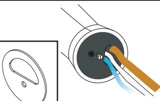
Make sure to use fiber gasket to ensure proper seal.
