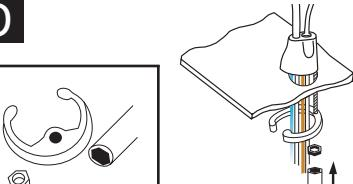
Semi-circular mounting plate should encircle all descending tubes and extend beyond sink hole when tight.
