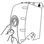
Mount tank vertically in an area that allows clearance on the underside of the tank for drainage, if necessary.
