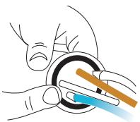
Make sure to use rubber O-ring to ensure proper seal.
