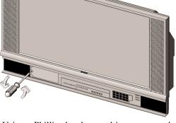
**3.** Using a Phillips head screwdriver, remove the screw securing the lamp cover; remove the cover.
