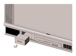
**5.** Remove the lamp unit from the television by grasping the handle and pulling it out. Dispose of lamp in accordance with local environmental regulations.
