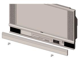
**9.** Replace the front cover by aligning it on the television and pushing gently until it snaps into place. Plug the power cord back into the wall outlet and turn on the power.
