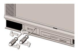
**4.** Remove the two screws on the lamp unit.
