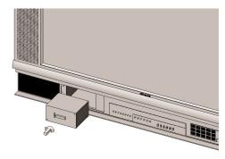
**6.** Insert the new lamp unit, paying attention to the orientation and direction of insertion. Ensure that the new unit is firmly seated.
