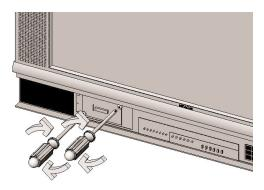
**7.** Tighten the screws firmly on the new lamp unit, taking care not to overtighten.
