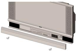
**2.** Remove the front cover of the television by pulling it outwards until the snap unlatches.
