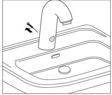
Block the sensor for 2 seconds.
