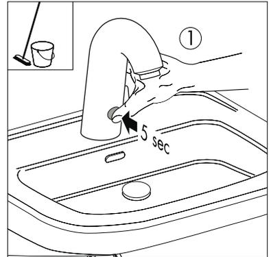
This will turn the water off for approximately 75 seconds so that the sink may be cleaned (2).
