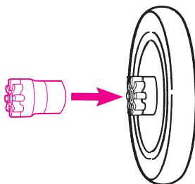
Firmly attach hub adapter onto wheel.
