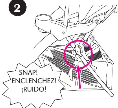
**CHECK** that the stroller is completely latched open before continuing.
