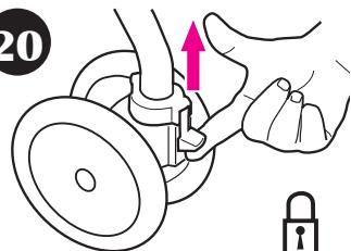
Front swivel wheels lock for use on uneven surfaces such as grass, stones or gravel.
