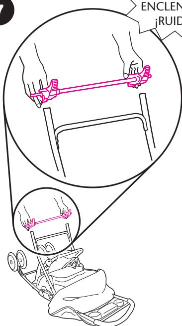
Brake levers point toward rear of stroller. **Check** that rear axle is securely attached by pulling on brake assembly.
