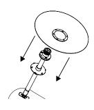
3. Firmly push the cover ring onto the securing collar snap clips until each clip snaps into place.
