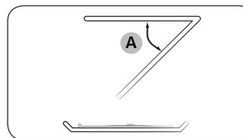
To clean the upper area of the cooking cavity lower the top heating element by 45° (A) as shown. This will help clean the upper area. When done, reposition the top heating element.
