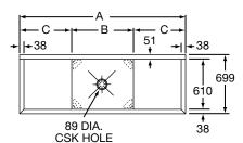
INDICATE NUMBER OF FAUCET HOLES WHEN PLACING ORDER. (NON-STANDARD FAUCET AND OVERFLOW DRILLING LOCATIONS ARE AVAILABLE. SPECIFY ON DRAWING AT RIGHT.)
