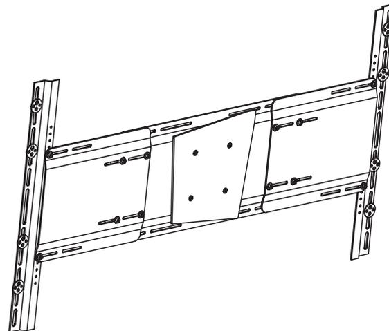
**FPD Adapter (for mounting Flat Panel Displays)**
