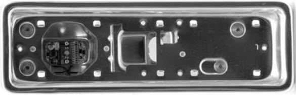
7. Feed the wires through the larger hole in the mounting plate and guide it to the bottom of the housing. The flat side of the mounting plate should be on the outside of the housing and the side with the slight raised center should go toward inside of the housing. This will properly align the mount in the original housing.
