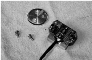
6. Insert the new LED assembly into the taillight housing and route wires through the hole where the original bulb and connector were located. Use caution when feeding the wires through to
