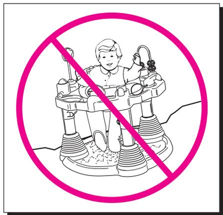
To avoid tipovers, place product on flat, level floor/ground. Adjust legs to same height so that the tray is level before placing child in product.
