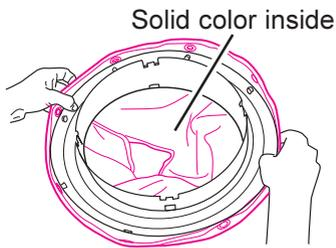
Attach the seat to the seat ring by tucking the seat edge into the channel and snapping the grommets on the pegs.
