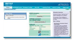
You can get back to the Setup page from anywhere in the configuration screens by clicking on the *Setup* tab in the top left corner. From here, you can rerun the Internet Connection Wizard, change your router mode, initiate AOSS or WPS, and see your wireless SSID and encryption settings.
