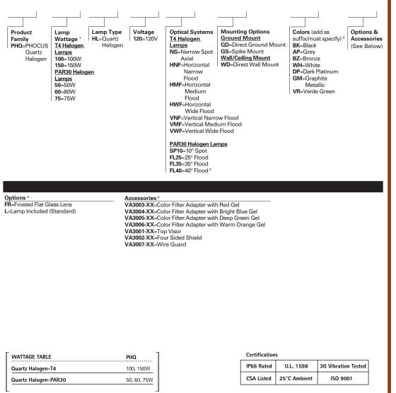
NOTES: 1 T4 lamps feature a mini-can base, PAR30 lamps feature a medium screw base. 2 60W PAR30 halogen lamp not available in FL40 distribution. 3 Custom and RAL color matching available upon request. Consult your INVUE Lighting Systems Representative for further information. 4 Add as suffix in the order shown. 5 Order separately, replace XX with color suffix. 6 Specifications and dimensions subject to change without notice.
