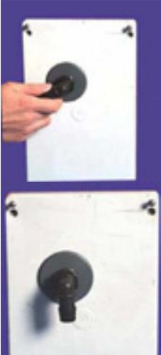
D.3.4 Screw in the black nylon 90° hose barb fitting and align the barb end such that it is pointing down.
