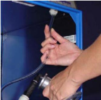
C.15 Initial Operation - Once the installation of the exhaust tubing is complete, ensure that the purge tube is connected inside the cabinet. The purge tube connects the sterilizer via an acetyl quick connect fitting that is located on the front right corner of the lower cabinet's ceiling. Check to make sure the power cord is connected to the back of the sterilizer and is plugged into an un-switched, grounded power outlet.
