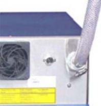
D.3.5 Take one end of the eight foot length of 3/4" (1.9 cm) I.D. clear braided PVC tubing and slip one of the stainless steel hose clamps over the end. Next, push the tubing as far as it will go onto the 90 degree hose barb connector on the back of the cabinet. Then secure the PVC hose by tightening the stainless hose clamp with a flat blade screw driver.
