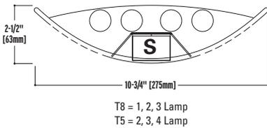
**Construction:** Housing is one-piece, die-formed, cold rolled steel, forming a 10-3/4" x 2-1/2" curved architectural profile. Perforated sections are 33% open with staggered hole pattern and opal diffuser. Standard 4'-0", 8'-0" and 12'-0" luminaire lengths combine for continuous runs.
