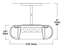
**Construction:** Formed 20-gauge cold rolled steel with internal structural bracing. Nominal 3', 4', 6' or 8' illuminated sections.
