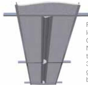
Recommended distance from fixture longitudinal axis and wall is 1' to 3'. Optimum performance distance is 2'. Not recommended for use outside this range. Fixture housing lengths are 3', 4' and 5' mounted individually in grid ceilings and in sheet rock. Can be mounted in continuous rows.
